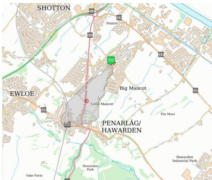
Figure 4: local catchment data shown on the FEH web service, showing the site sits within a localised catchment discharging to the ordinary watercourse.
