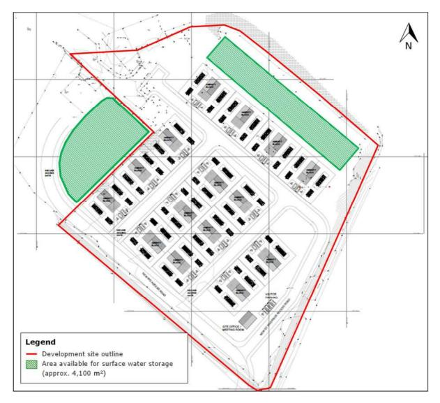
Figure 9: Preliminary Surface Water Drainage Layout
