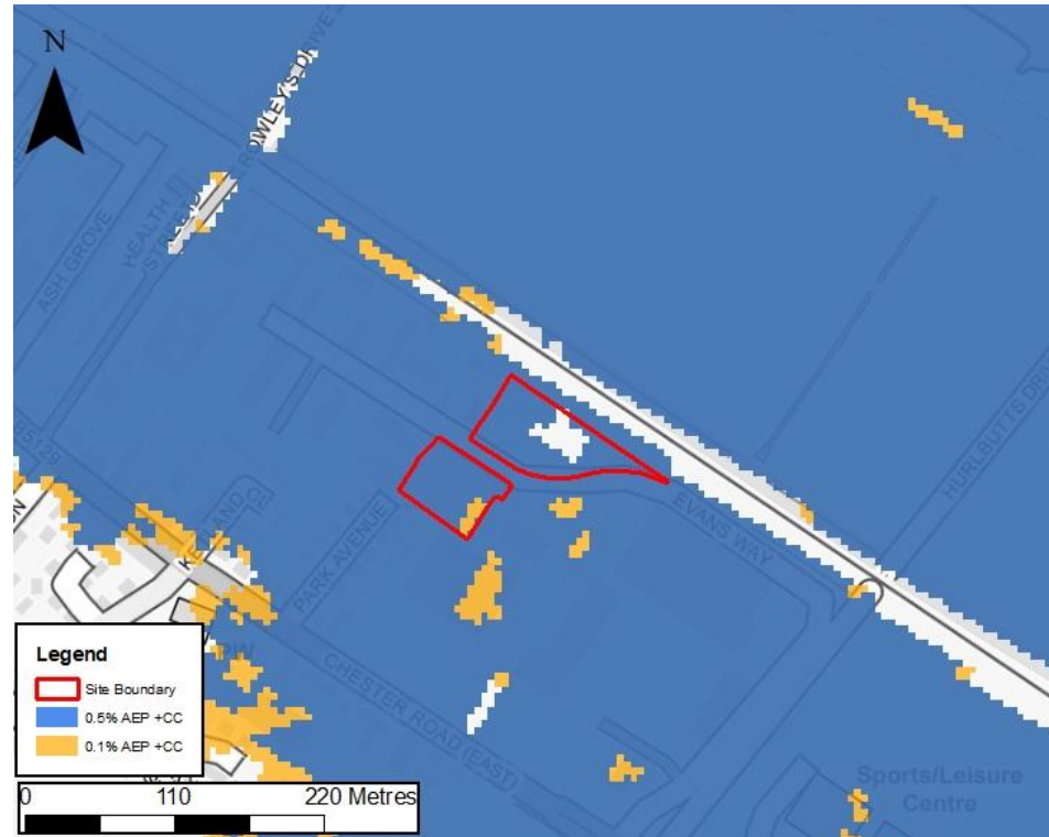
Figure 9-17 Modelled Queensferry breach flood extents for the 0.5% AEP +CC and 0.1% AEP +CC events
