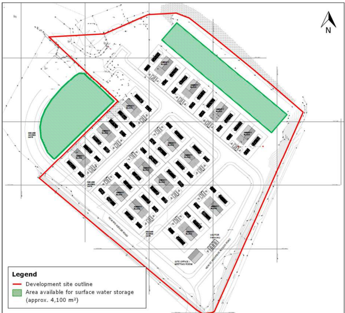
Figure 9: Preliminary Surface Water Drainage Layout
